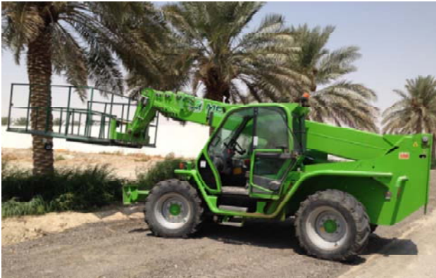
Truck mounted platform to perform operations in the crown of date palm
