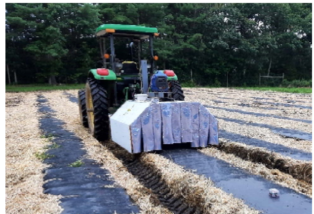
Fig. 1 : (Left) Cutaway end view of the UV-C enclosure showing placement of the fixtures. (Right) UV-C treatment attachment mounted to a tractor and shown positioned over an unplanted row.
