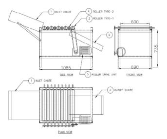
Fig. 2. Diagram of onion detopping machine all dimensions in mm
