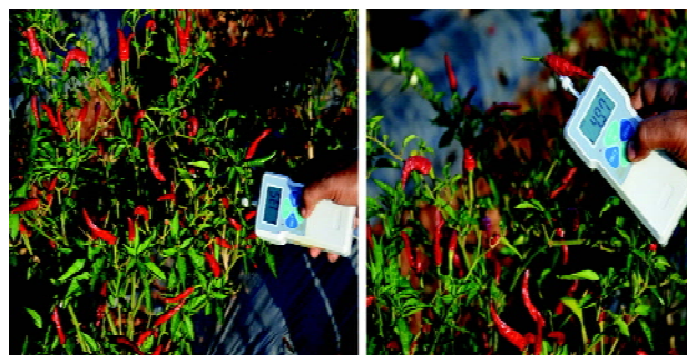
Fig. 2. Images showing fruit detachment force with digital force gauge
