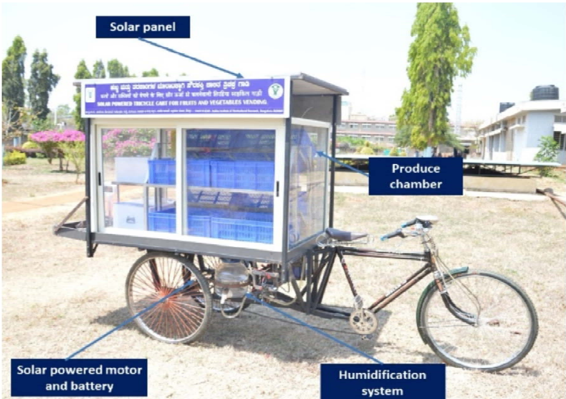
Solar power operated tricycle cart for fruits and vegetable vending
