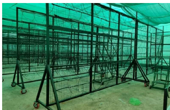
Fig. 3 : Vertical frames (left) and horizontal benches (right) used for cultivation
